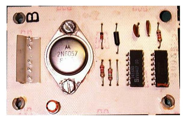
This is a picture of the pop bumper driver board before I rebuilt it. You can tell by the orientation of the black tantalum capacitor (C3) and the single 1N4148 diode that this board is the modified version.
